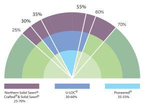
Vintage's Crafted® hardwood flooring is designed for areas requiring a thinner construction 1/2". Crafted® will perform well if humidity levels are maintained with warranty limits. If floors are exposed to relative humidity conditions higher or lower than warranty limits for extended periods of time, tenting or panelization are potential issues, respectively. This is especially relevant when floating the floor.
